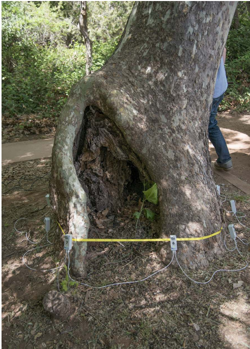
ARBOTOM® - sonic (stress wave) line tomogram:
